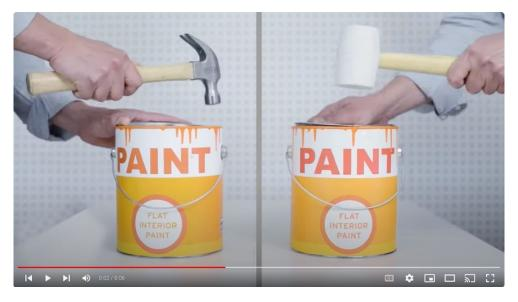
Examples of Storage Tip Video Showing Use of a Rubber Mallet to Avoid Damaging Can
