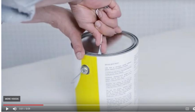
Example of Storage Tip Video Showing Use of a Paint Can Key to Avoid Damaging Can
