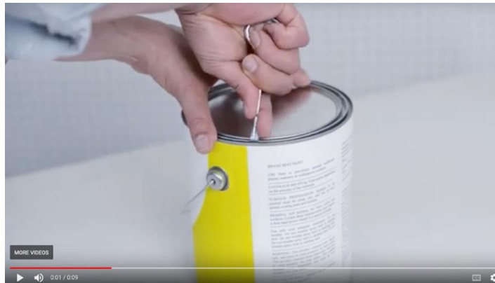
Examples of Storage Tip Video Showing Use of a Paint Can Key to Avoid Damaging Can
