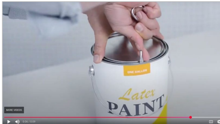
Example of Storage Tip Video Showing Use of a Paint Key or Paint Can Opener to Avoid Damaging Can
